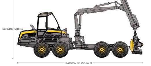
GRAPPLE Model: Several different grapple alternatives LOAD SPACE 14 000 kg (30,865 lb) Capacity: 15 000 kg (33,069 lb) with balanced bogies Load space cross-sectional area: 4,5–5 m<sup>2</sup> Load space length: 4 100-4 650 mm (161-183 in) + glide bunk 700 mm (28 in) Log gate can be moved hydraulically.
